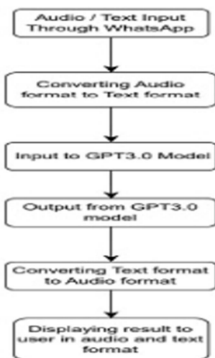
Drawing 1 of 2: System Architecture of WhatsApp Chatbot Powered by ChatGPT for Medical Advice in Indian Regional Language
