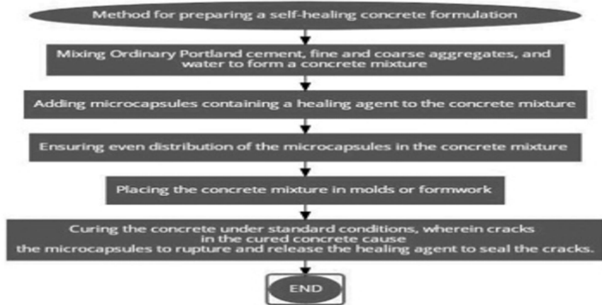
Fig. 1 A method for preparing a self-healing concrete formulation
