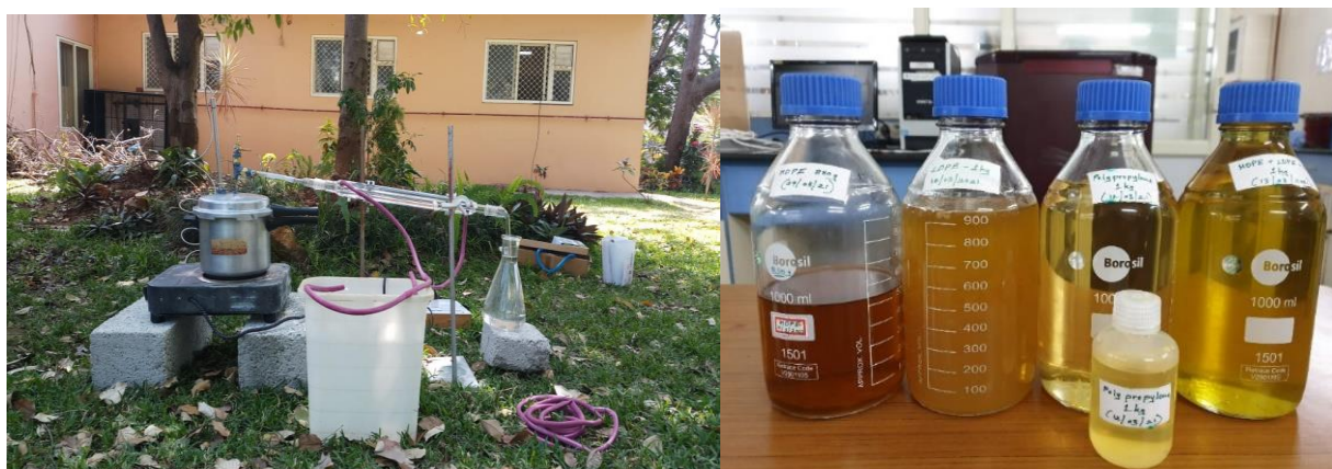
Plastic pyrolysis reactor and the products generated from it.
