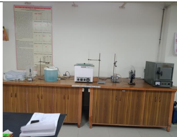
Complete lab setup for measurement of Ultrasonic velocity, density, viscosity and refractive index at varying temperature and concentrations,
