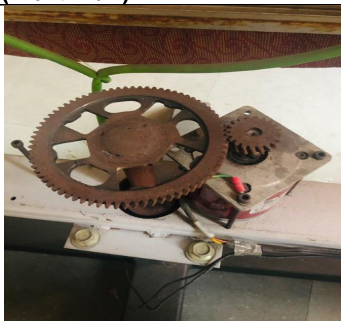
Mechanical Gear attached to stepper motor
