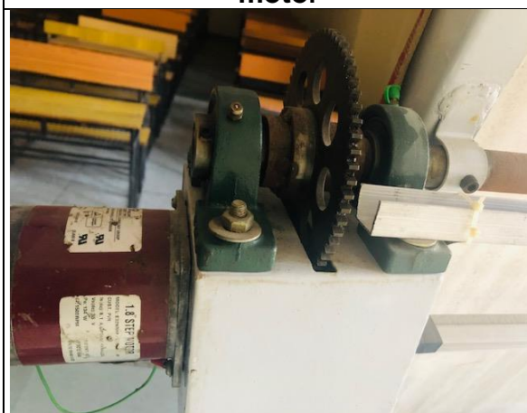
Mechanical Gear attached to stepper motor
