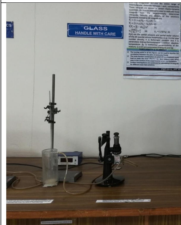
Left to right: 1. Double walled glass jacket to maintain the temperature by putting pycnometer and Ostwald Viscometer for density and viscosity of pure, binary and ternary mixtures at varying temperatures
