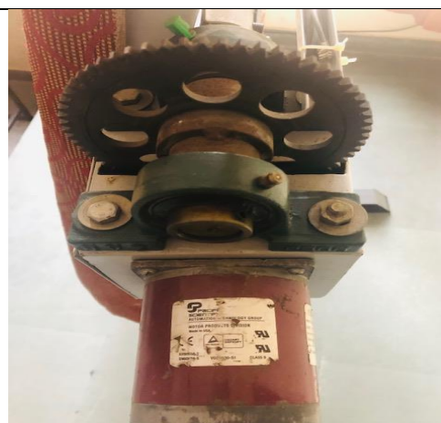
Stepper motor attached to both ends of the mechanical gear system
