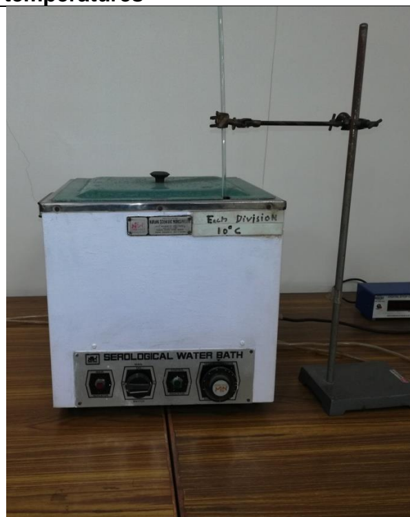
Water Bath: to increase the temperature above to room temperature
